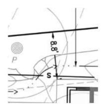
Note: Common <u>zoning laws</u> define eave lines to be "The lower edge of a sloping roof that projects past the face of the wall." Architecture drafting programs can automatically display these lines as shown in the diagram above.
